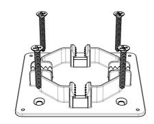
Screws may require additional fixing accessories like wall plugs for masonry.
