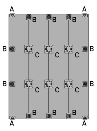
The clips supplied are appropriate for the installation of 6 tiles arranged in a  $3 \times 2$  grid. The arrangement above can be achieved with 2 boxes (12 tiles). Other layouts will require extra clips.
