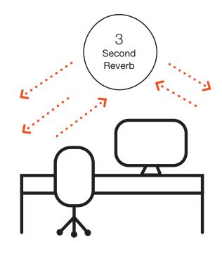
KnollTextiles *Impressions* acoustic tiles have an overall NRC of 0.55 while providing almost perfect absorption (0.77 -0.93) at the frequencies where the human voice registers (1,000-2,000 Hz). This means the tiles are highly effective at absorbing the sound of voices and reducing the reverberation time (the amount of time it takes for sound to dissipate) in an interior space.
