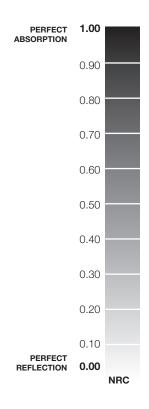
Another method of measuring sound absorption is the Sound Absorption Average (SAA). The SAA is identical to NRC, except that twelve one-third octave measurements, from 200 Hz to 2500 Hz, are averaged instead of the four used to ascertain an NRC rating. The other difference is that NRC results are rounded to the nearest 0.05 and SAA results are not.
