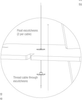
**Step 7**Adjust cables to desired length via squeeze clutch within cable support and cut/remove excess cable
