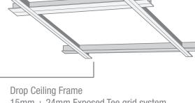
15mm + 24mm Exposed Tee grid system [ Not supplied ]
