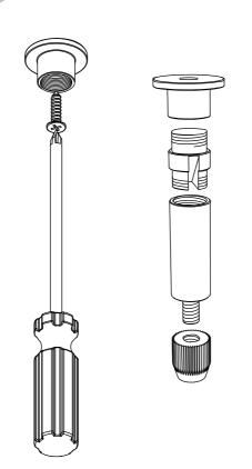
Feed the cable through the panel fixture first, then through the panel fixture cover.
