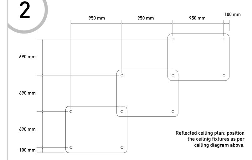
If feeding the cable through a panel is required, pop out cutouts to reveal 8mm holes, these are inset 100 mm from the corners of the pa nel.
