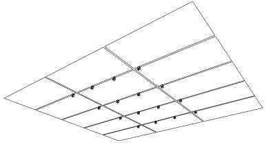
Slot top and bottom blades together forming a square grid.
